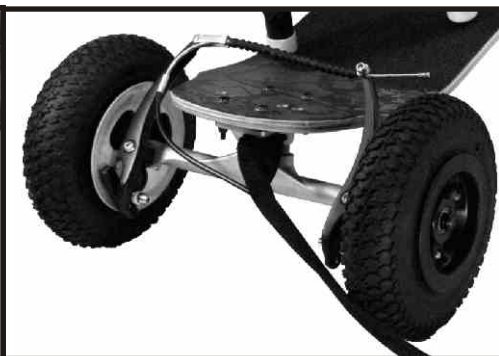
BRAKE ASSEMBLED ON ATS TRUCK
